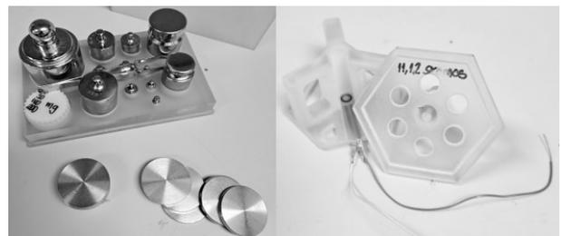
Fig.3. Weight kit and sensor support.
