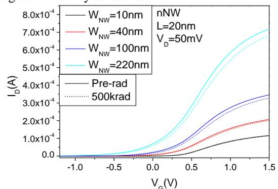
Fig. 2. Drain current as a function of gate voltage for four different width (20nm, 40nm, 100nm and 220nm) to n-channel devices.
