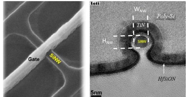
Fig. 1. (Left) SEM and (right) cross-sectional TEM images of  $\Omega$ GNW MOSFETs with an 8-nm diameter.
