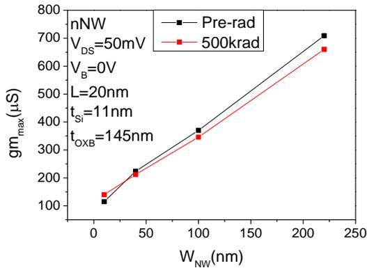
Fig. 4. The value of the maximum transconductance as a function of width for the devices, before and after proton radiation.
