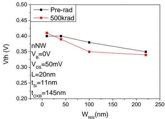
Fig. 5. The value of the threshold voltage as a function of width for the devices, before and after proton radiation.
