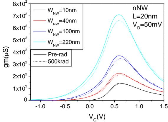
Fig. 3. The transconductance as a function of gate voltage for four different width (20nm, 40nm, 100nm and 220nm) to n-channel devices.
