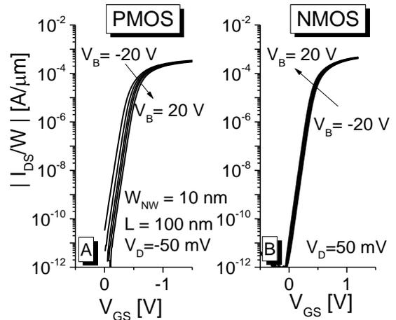
Fig 2 - Normalized by  $W_{NW}$  drain current of  $\Omega$ -Gate NW for width of 10 nm on pMOS device (A) and nMOS (B) for different back gate bias ( $V_B$ ).
