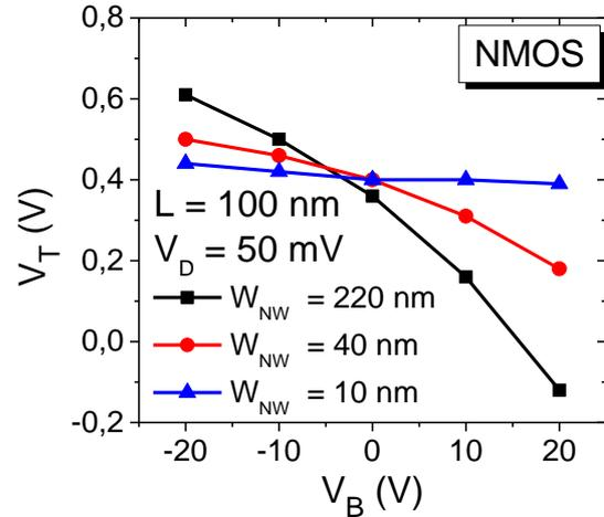
**Fig 5** - Threshold voltage as a function of back gate bias for different channels widths on nMOS devices.
