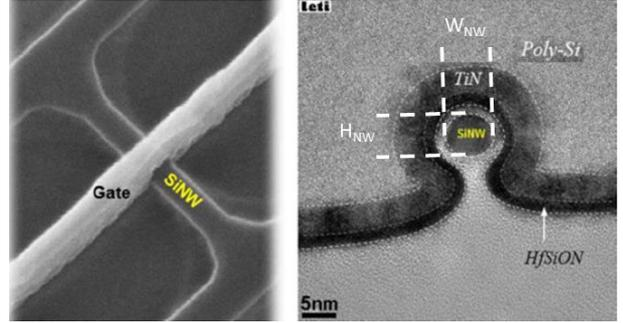
Fig 1 - (Left) SEM and (right) cross-sectional TEM images of SOI Omega-Gate Nanowire [1].
