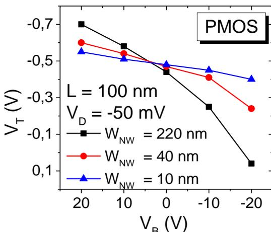
**Fig 4** - Threshold voltage as a function of back gate bias for different channels widths on pMOS devices
