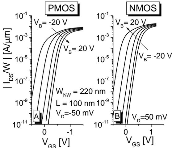
**Fig 3** – Normalized by  $W_{NW}$  drain current of  $\Omega$ -Gate NW for width of 220 nm in pMOS device(A) and nMOS (B) for different back gate bias ( $V_B$ ).
