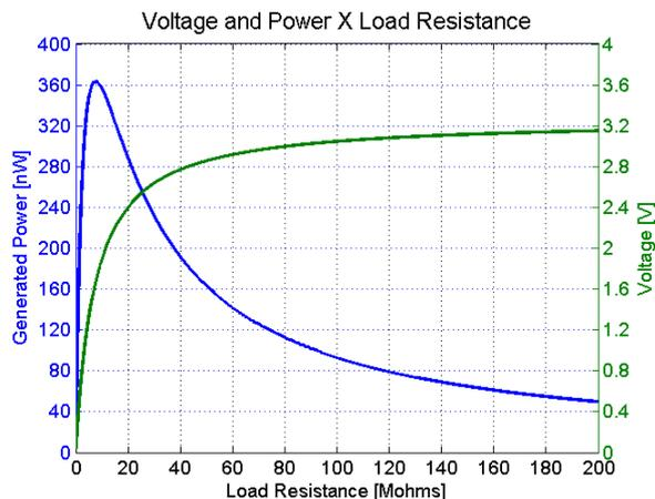
**Fig.2.** Plot of generated power and voltage vs load resistance for ambient vibrations of 4m/s<sup>2</sup> of intensity in 147.41Hz.
