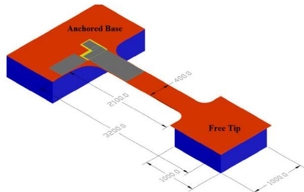
Fig.1. Device structure with dimensions in  $\mu$ m.
