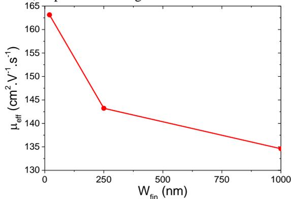
**Fig.4.** Calculated mobility as a function of the fin width
