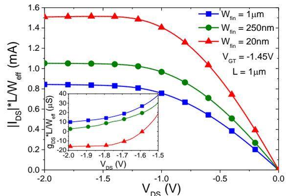
Fig.2. Normalized drain current as a function of the drain voltage varying the fin width for a channel length of  $1\mu\text{m}$
