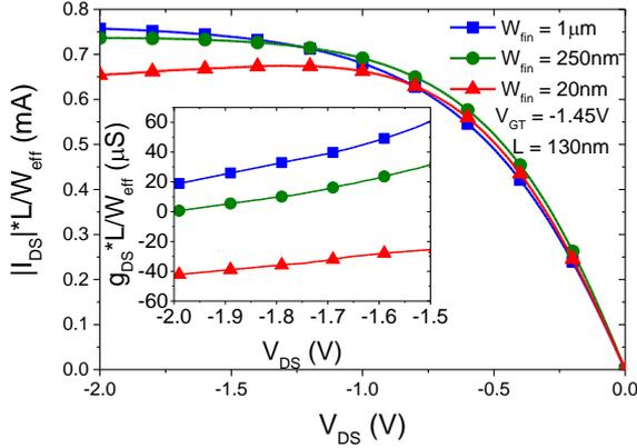
**Fig.3.** Normalized drain current as a function of the drain voltage varying the fin width for a channel length of 130nm
