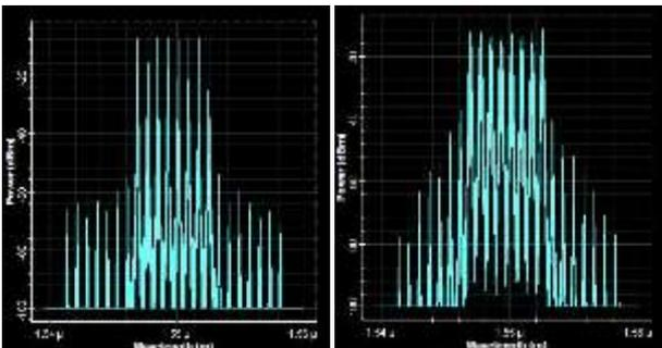
Fig. 3. Optical Spectrum at Fiber Output When Input Power is 13 dBm (left) and 20 dBm (right).
