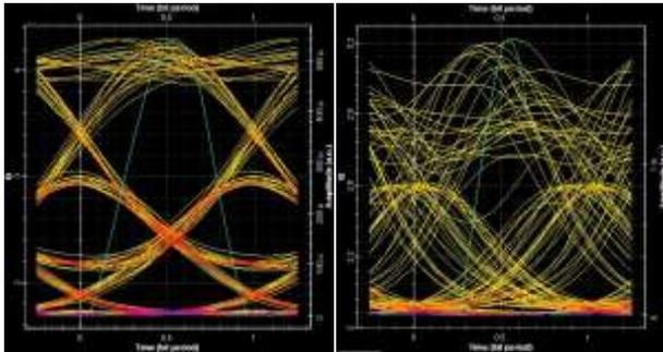
Fig. 2. Eye diagrams Cross-phase modulation for 0 dBm (left) and 16 dBm (right).
