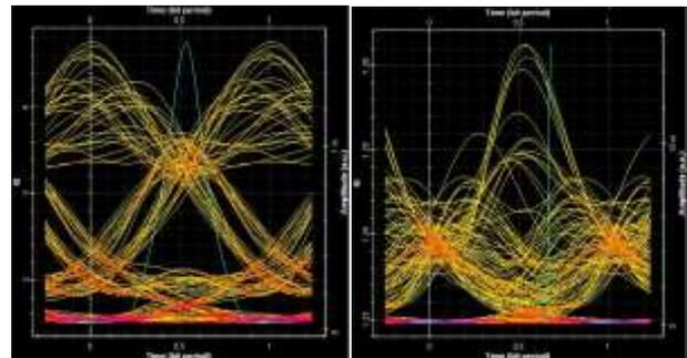
**Fig. 1.** Eye diagrams for Self-Phase Modulation for -10 dBm (left) and 10 dBm (right) Input.
