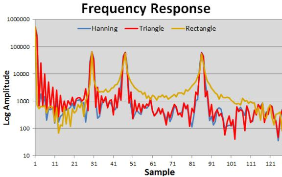
Fig. 3 shows the frequency response of the same signal, with four frequency components combined, while applying different windowing techniques.
