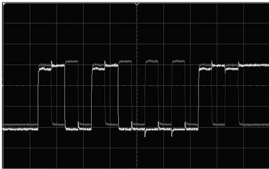
**Fig.2.** SPI communication: sending A3h to write in register. The gray waveform is SCLK, while the white waveform is MOSI.
