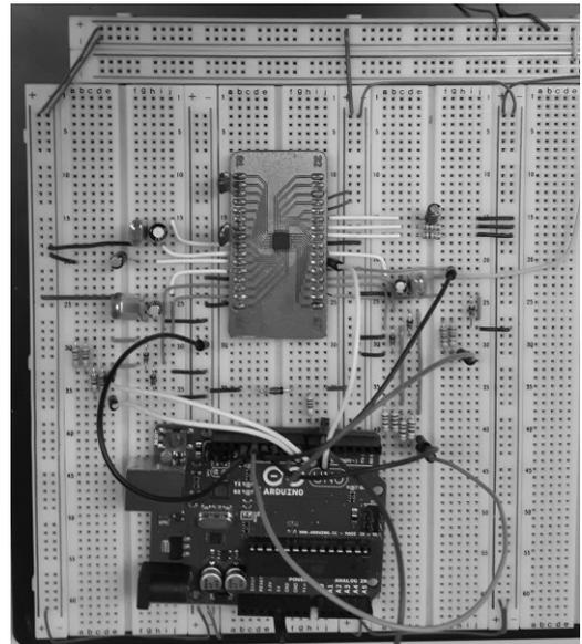
**Fig.3.** Hardware for initialisation of ADS1292 using the Arduino Uno board.
