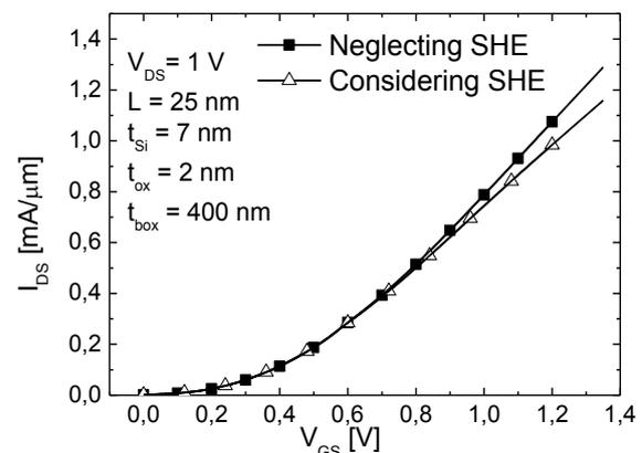
**Fig.1.** Drain current ( $I_{DS}$ ) as a function of the gate voltage ( $V_{GS}$ ) for  $V_{DS} = 1$  V demonstrating the degradation due to the self-heating effect.
