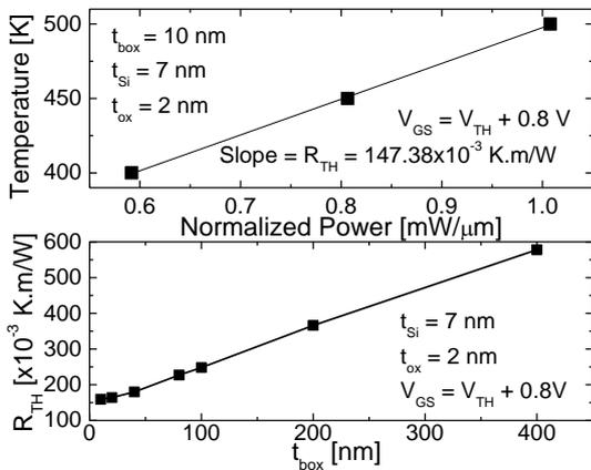
Fig.3. Device temperature as a function of the normalized power for a 400 nm- $t_{box}$  transistor (top) and thermal resistance as a function of  $t_{box}$  for different devices.
