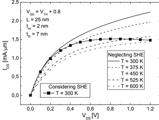
Fig.2. Drain current as a function of the drain voltage considering and neglecting SHE for the application of the Hot Chuck method.
