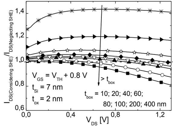
Fig.4. Ratio between the drain current considering and neglecting the SHE ( $I_{DS(Considering\ SHE)} / I_{DS(Neglecting\ SHE)}$ ) as a function  $V_{DS}$  for devices with different buried oxide layers.
