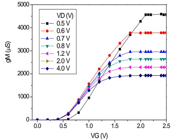
**Fig.4.** Transconductance (gM) as a function of gate voltage (VG) for SOI UTBOX nMOSFET.
