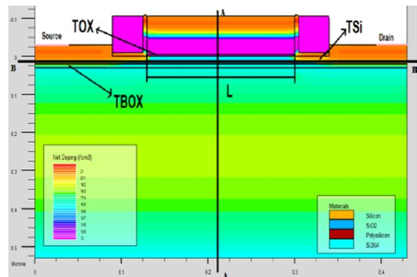
**Fig.1.** SOI UTBOX nMOSFET net doping indicating Source, Drain, line A–A, line B–B and different parameters like TOX, TSi and the channel length (L).
