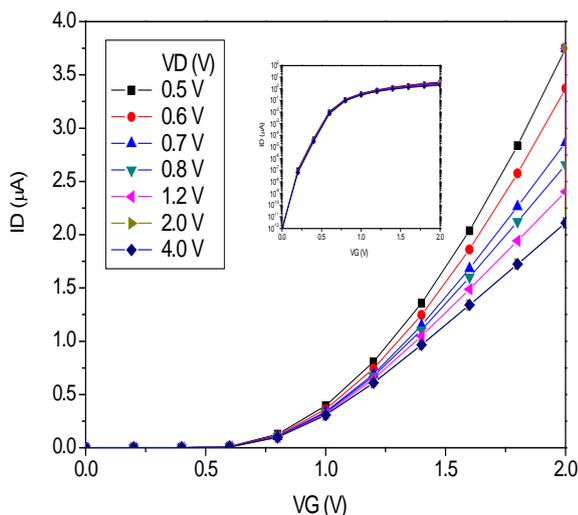
**Fig.3.** Drain current (ID) as a function of gate voltage (VG) for SOI UTBOX nMOSFET.
