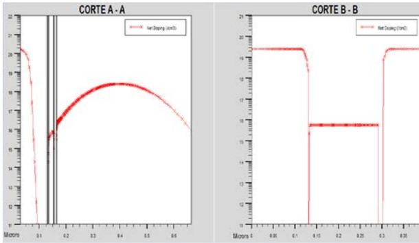
**Fig.2.** Doping Concentration as a function of length (line A–A, line B–B indicating in Fig.1).
