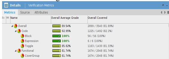
Fig. 3. Code and Functional Coverage
