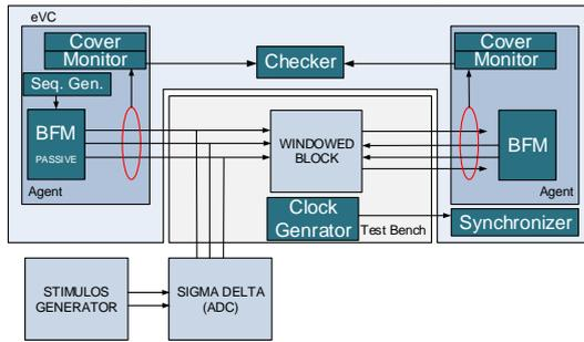
Fig. 2. Verification Architecture
