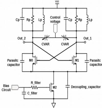
**Fig.2.** Cross-Coupled VCO schematic
