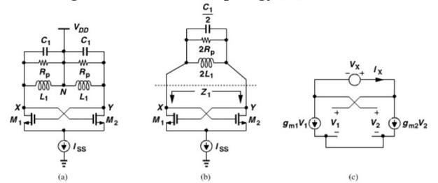
**Fig.1.**(a) Redrawing of cross-coupled oscillator, (b) load tanks merged, (c) equivalent circuit of cross-coupled pair
