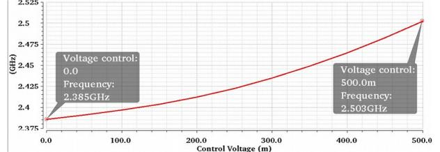
**Fig.3.** Frequency oscillation controlled by voltage
