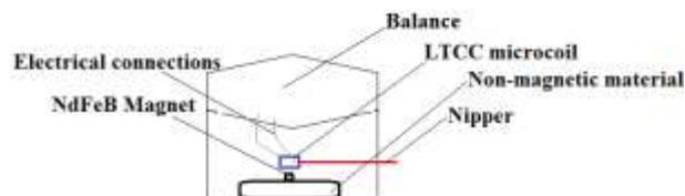
**Fig5.** Schematic representation of the experimental setup used to measure the force produced by the coil over the magnet.
