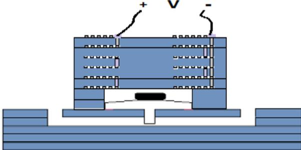
**Fig.1.** Concept of the electromagnetic LTCC-PDMS microvalve.
