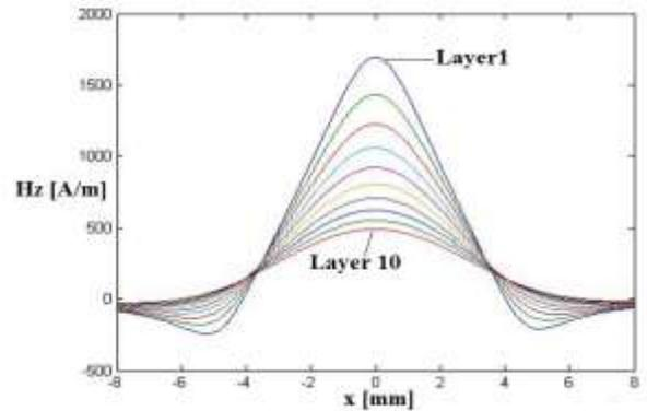
**Fig.3.** Magnetic field  $z$  component simulation produced by each layer of a three-dimensional coil with 10 flat layers ( $n = 94$ ,  $g = 200 \mu\text{m}$ ,  $I = 0.55\text{A}$ ,  $y = 0 \text{mm}$ ,  $z = 1 \text{mm}$ ).
