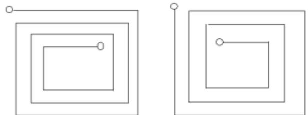
**Fig.4.** Schematic representation of the layers used to fabricate the windings on the surface of LTCC sheets.
