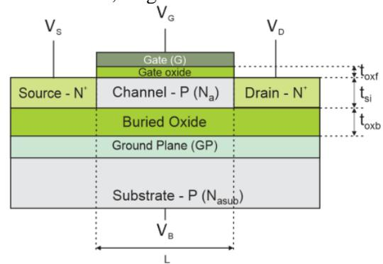
Fig. 1. A schematic cross-section of an UTBOX/UTBB SOI device with GP.
