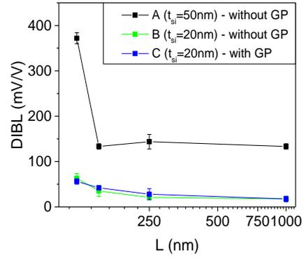
Fig. 5. Experimental curve of DIBL as a function of channel length.
