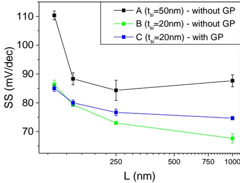
Fig. 3. Experimental curve of subthreshold swing as a function of the channel length.
