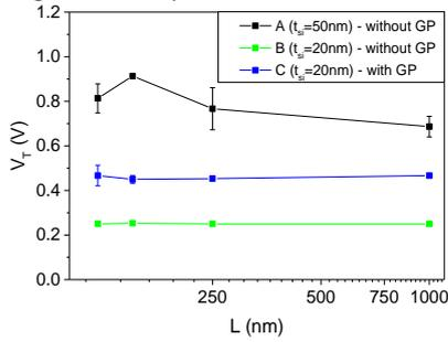
Fig. 2. Experimental curve of threshold voltage as a function of the channel length.
