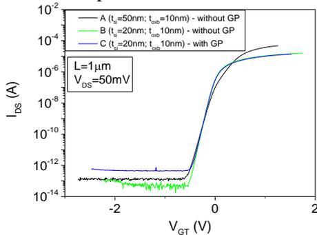
Fig. 4. Experimental curve of drain current as a function of gate overdrive voltage.
