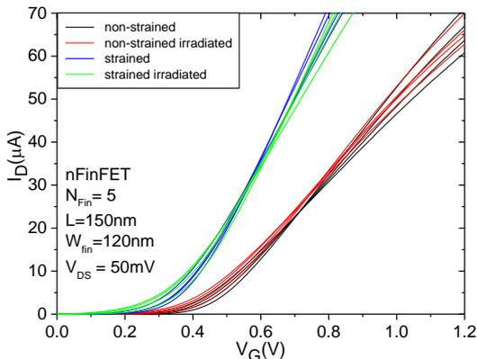
**Fig 4** - Experimental drain current ( $I_D$ ) in function of gate bias ( $V_G$ ) for different temperatures for non-strained and strained, non-irradiated and irradiated devices in the linear region.
