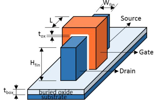
Fig 1 - A tri-dimensional schematic view of a triple gate SOI FinFET.
