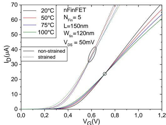
**Fig 3** - Experimental drain current ( $I_D$ ) in function of gate bias ( $V_G$ ) for different temperatures for non-strained and strained, non-irradiated devices in the linear region.
