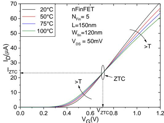
**Fig 2** - Experimental drain current ( $I_D$ ) in function of gate bias ( $V_G$ ) for different temperatures for non-strained and non-irradiated devices in the linear region.
