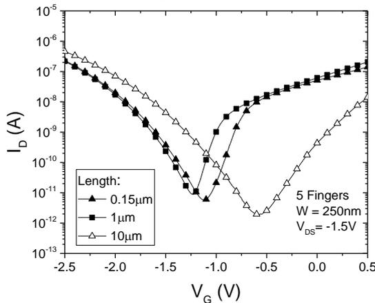
**Fig.3.** Drain current as a function of gate voltage for different lengths of 250 nm channel width p-TFET devices.
