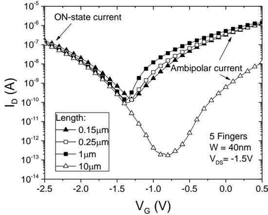
**Fig.2.** Drain current as a function of gate voltage for different lengths of 40 nm channel width p-TFET devices.
