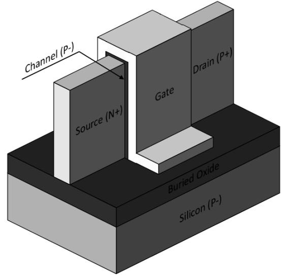
*Fig.1. Self-aligned triple gate SOI p-TFET simplified diagram.*
