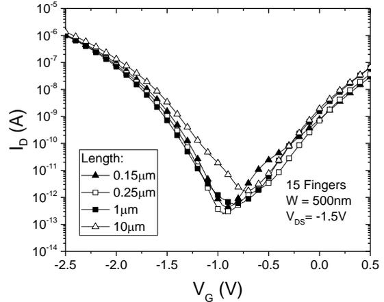
**Fig.4.** Drain current as a function of gate voltage for different lengths of 500 nm channel width p-TFET devices.
