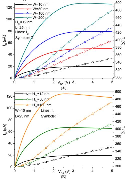
**Fig.2.** Drain current and lattice temperature as a function of drain voltage for different channel widths (A) and fin heights (B).
