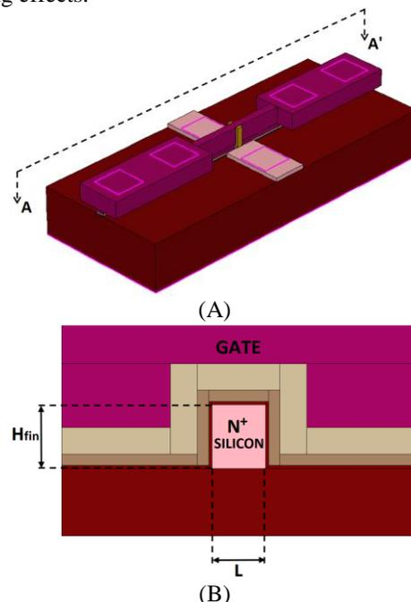
Fig.1. Three-dimensional scheme (A) and longitudinal (B) section of the simulated device.
