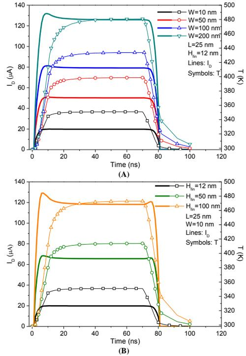
**Fig.3.** Drain current and lattice temperature transient for different channel widths (A) and fin heights (B).
