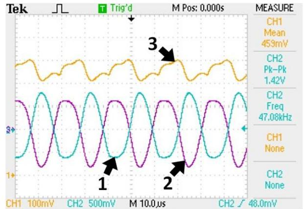
Fig. 4. Voltage waveforms for the circuit with one feedback loop:  $L_6$  (1),  $L_7$  (2),  $V_B$  (3).
