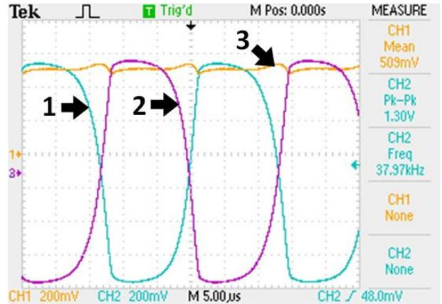
Fig. 3. Voltage waveforms for the circuit with two feedback loops:  $L_6$  (1),  $L_7$  (2),  $V_B$  (3).
