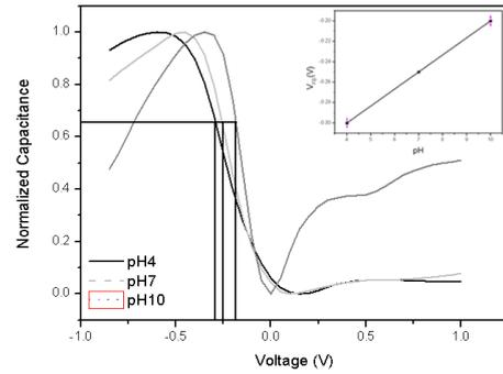
**Fig 3.** Normalized  $C_xV$  curve for each pH value. The inset shows  $V_{FB} \times \text{pH}$  curve.
