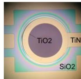
**Fig.1.** Electrolyte-Insulator-Semiconductor with TiN as reference electrode.
