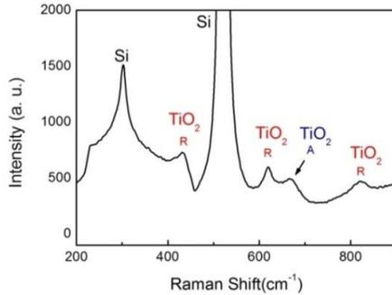
**Fig.2.** Raman spectrum of the  $\text{TiO}_2$  film.
