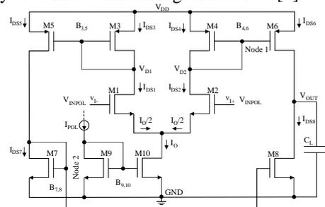
Fig.1. Schematics of the single-stage single-end OTA used in this work.
