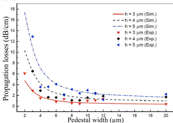
**Fig.4.** Simulated and experimentally measured propagation losses for waveguides with pedestal height of 3, 4 and  $5\ \mu\text{m}$  and widths ranging from 2 to  $20\ \mu\text{m}$ .
