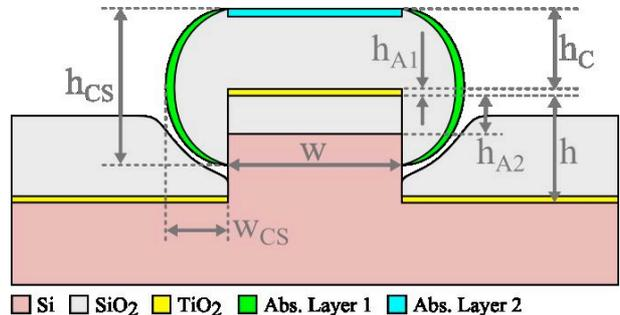
**Fig.1.** Waveguide cross-section model used in the FDM simulations.
