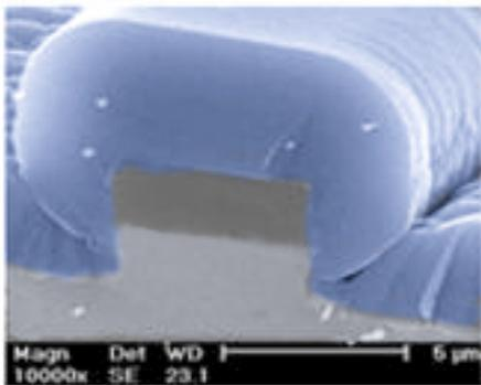
**Fig.3.** SEM micrographs of pedestal ARROWs with pedestal height  $h = 4\ \mu\text{m}$ .
