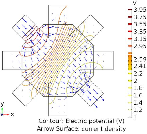
Fig. 2. Simulated current flow and equipotential lines distorted due stress
