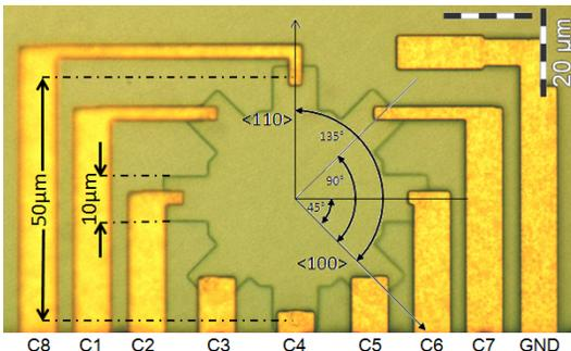
Fig. 1. Eight Terminal Silicon Piezotransducer (8TSP)
