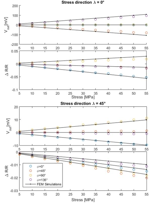
Fig. 3. Comparison between experimental measures (round circles) and FEM Multiphysics simulation results (straight black lines)
