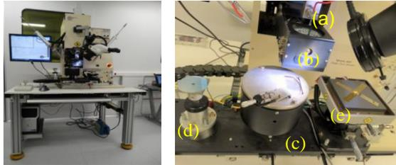
**Fig. 2.** Eagle 860 Omni Bonder equipment and some details of it.
