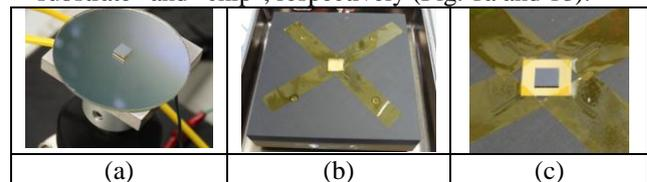
*Fig. 1. (a) Chip on the Pick up Stage, (b) Substrate on the Work Stage, (c) Chip flipped and bonded onto the substrate*
