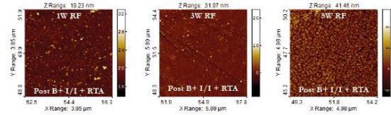
Fig. 3: AFM Images of the film surfaces after B<sup>+</sup> I/I RTA.
