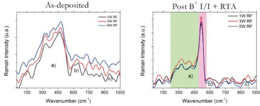
Fig. 2: Raman spectra of the films as-deposited left and post B<sup>+</sup> I/I RTA in the right. The areas under the spectra shows: a) Si-Si vibration modes, b) and c) Si-H vibration mode at  $620\text{ cm}^{-1}$  and  $950\text{ cm}^{-1}$ , respectively.
