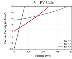
Fig. 4: IV curves of the amorphous/silicon (a-Si:H/C-Si) heterojunction (SHJ) solar cells illuminated (with AM 1.5) conditions.
