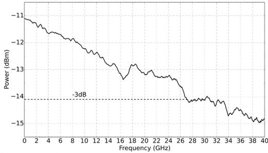
Fig 5. Photodetector O-E bandwidth
